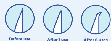
Pen needle wear after use
