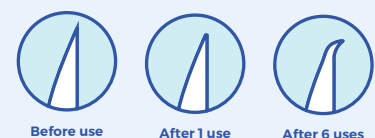
Pen needle wear after use
